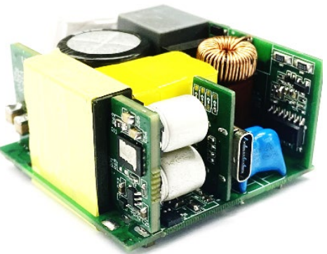
~750 kHz peak Half-Bridge GaN IC 120 W, 44 cc
