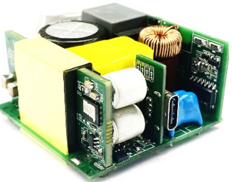
~750 kHz peak Half-Bridge GaN IC 120 W, 44 cc
