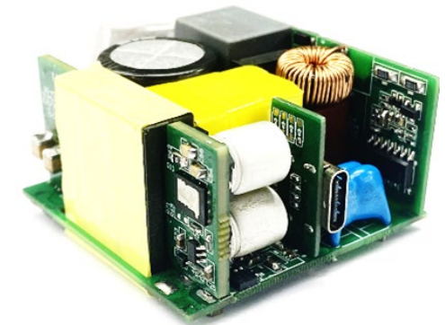
~750 kHz peak Half-Bridge GaN IC 120 W, 44 cc
